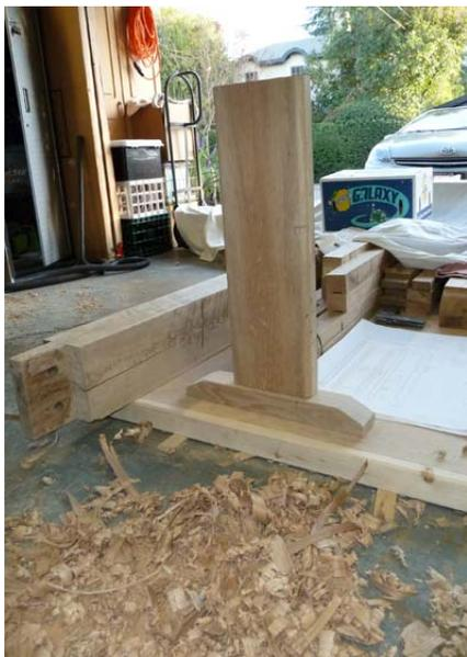
Not all of the work was done with saws, either. The forestay (in the photo at left) is made out of some kind of really hard, "Old Ironside" oak. When I tried to plane it to size, the plane just bounced off, no matter how sharp the blade, no matter the depth or the angle of the cut. As you can see from the chips on the floor, I wound up chiseling the wood to the thickness I wanted, then sanding it. Again, hard work.
